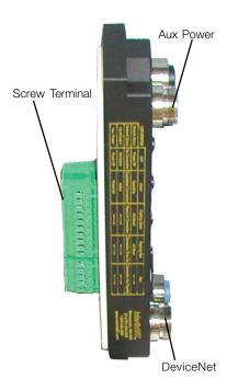
The FDNP-S0808G-ST *busstop®* station is designed to be mounted directly on motor control enclosures. Once mounted, the I/O, power and DeviceNet™ signals are available both inside the enclosure and outside the enclosure. Inside the enclosure the signals are accessed via removable screw terminals on the back of the station. Outside the enclosure the signals are accessed via *eurofast®* or *minifast®* connectors on the front of the station.
